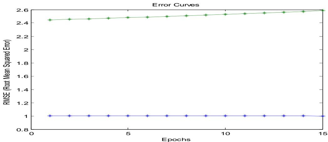
From this graph, it can be seen that the Root Mean Squared Error (RMSE) increases when epoch increases. To avoid overfitting problem, we set training epoch equals to twelve.
