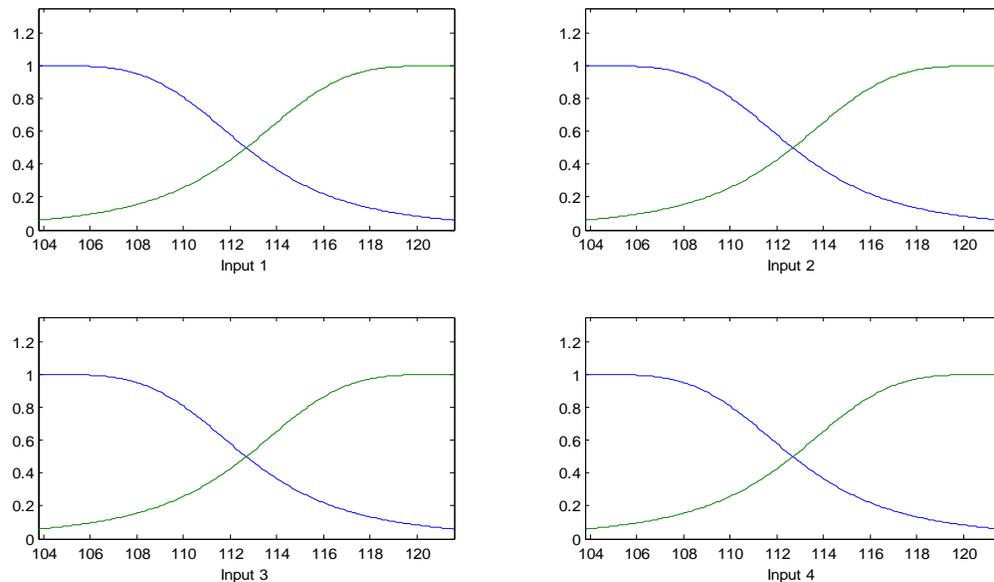
The initial MFs need to be trained by several epochs. The trained ANFIS model has 104 fitting parameters (see Appendix for details), including 24 nonlinear parameters which are optimized via back-propagation (3 parameters for each premise MF) and 80 linear parameters which are optimized via linear least-squares estimation (five parameters for each consequent equations). In order to achieve good generalization
